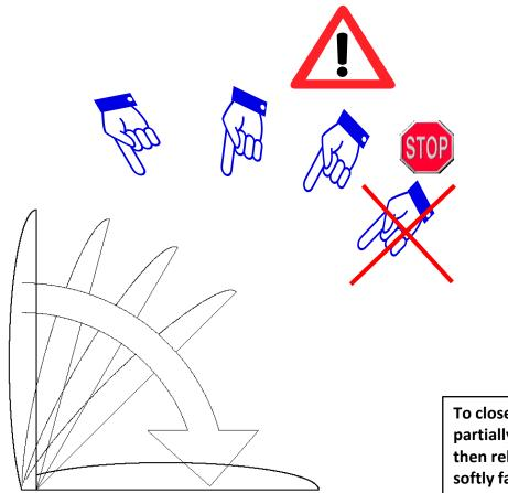
To close soft close seat partially close the seat, then release it. Seat will softly fall until closed.
